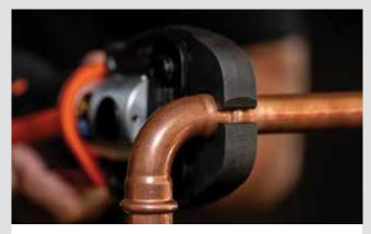
**8.** Initiate the pressing job by pressing the start button. The automatic pressing process guarantees a tight connection. The pressing process can be interrupted by pressing the emergency-stop button.
