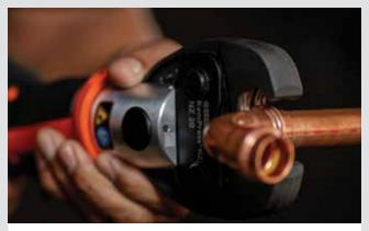
**7.** Check the fitting outer edge still lines up with the marking. Open the pressing jaw and close it around the fitting so the raised bump in the fitting rests inside the groove of the pressing jaw. Ensure the jaw is engaged square with the fitting and not on an angle.
