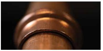
Unpressed fitting - small gap between fitting and tube.
