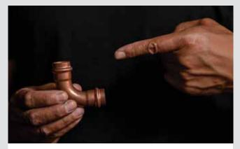
**6.** Ensure you have the correct fitting for the application (e.g. water or gas). Check the fitting is clean and the O-ring is free from debris and correctly sitting in place. Push fitting on tube all the way to the engagement marking.
