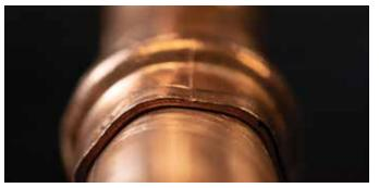
Pressed fitting - no gap between fitting and tube.
