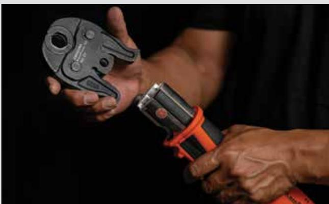
**5.** Select pressing jaw according to the fitting dimension and insert into the pressing machine. Arrest the locking bolts of the machine. Check the jaws are free from debris and in good working order.
