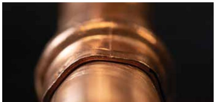
**Pressed fitting** - no gap between fitting and tube.
