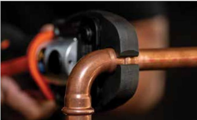
**8.** Initiate the pressing job by pressing the start button. The automatic pressing process guarantees a tight connection. The pressing process can be interrupted by pressing the emergency-stop button.
