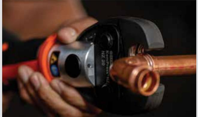
**7.** Check the fitting outer edge still lines up with the marking. Open the pressing jaw and close it around the fitting so the raised bump in the fitting rests inside the groove of the pressing jaw. Ensure the jaw is engaged square with the fitting and not on an angle.
