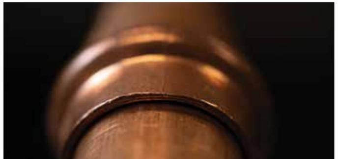
**Unpressed fitting** - small gap between fitting and tube.
