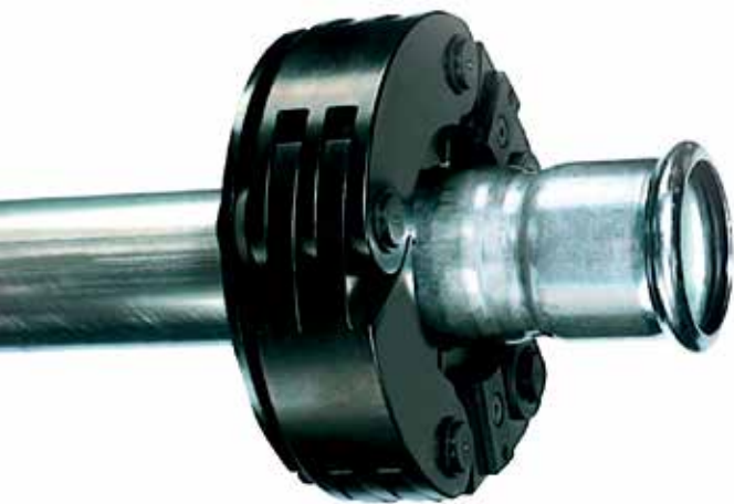
KemPress® Stainless fittings 76.1 mm and 108 mm do not have a leading lip prior to the O-ring.
